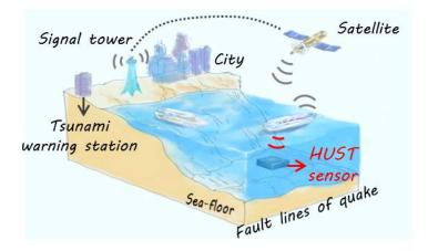
Schematic of Self-powered, Sea-water Based Electrochemical Underwater Pressure Sensors for 1mm to 30m Wave Monitoring and its perspective use in Tsunami Early Warning System Electronics Symposium
